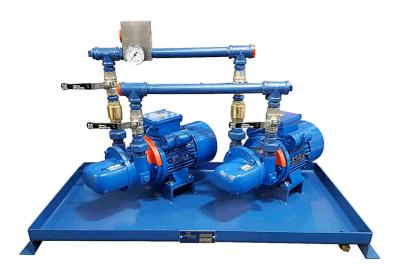
At the heart of these duty specific systems are the tried and tested NOV Mono M or G range pumps. The Mono pumps have no metal to metal wearing surfaces and incorporate a helical rotary action providing a low noise level, low power consumption, freedom from vibration and a self priming ability for over tank installation if required. This said, we can also specify alternate pumps for specialist applications.
